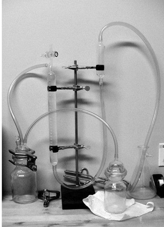
**Fig. 9.** Gas-collection apparatus for acid-digestion analysis based on the original design by H. Jedrzejewska as described in his 1960 article. Courtesy of Lori Aument, John Milner Associates, Inc.
