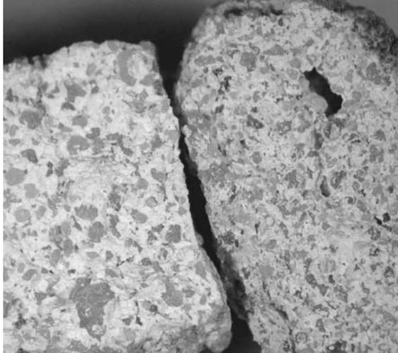
**Fig. 3.** Stereomicroscopic view of two mortar samples, 10x. Both of these samples are lime mortars of similar character, but differences between the binder aggregate ratios and aggregate size are easy to see. At higher magnifications, distinctive characteristics of the binder and voids are clearly visible.
