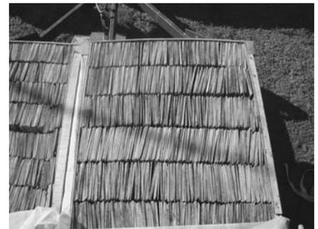
Fig. 10. A delivery crate packed tightly with banded bundles, arranged by size, of new red oak shingles for use at the Wright's Ferry Mansion, in Columbia, Pennsylvania.
