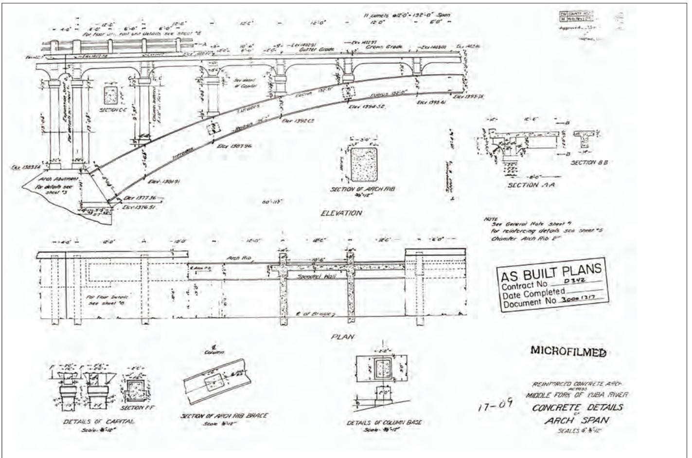
Fig. 4. Freeman's Crossing Bridge, Nevada County, California, construction documentation, 1920-1921, HAER CAL,29-SANJUN.V,1. This drawing shows a reinforced-concrete arch whose primary proportions were probably determined by appeal to empiricist formulas.
