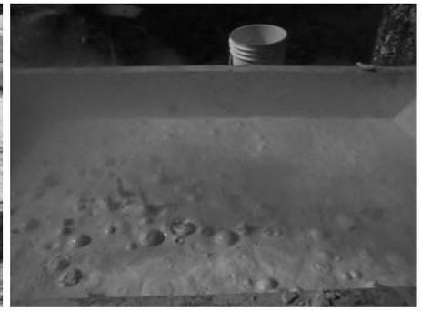
formed. The slaking process is an exothermic reaction, meaning that a great deal of heat is generated (Figs. 7 and 8):
