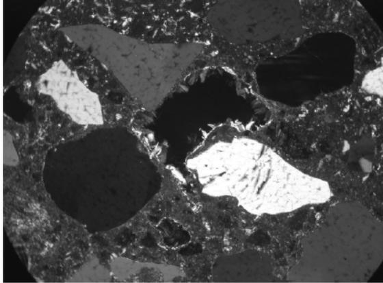
**Fig. 3.** View of a mortar sample in thin section, crossed polars, 400x magnification. Experience with a particular analysis method is critical to selecting proper sample-preparation procedures. Without proper sample preparation, the material lining the void in this sample would have been lost.
