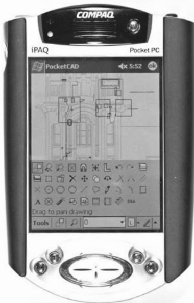
Fig. 1. Drawing-tool palette displaying a graphically annotated elevation using the PocketCAD/Compaq iPAQ system.
