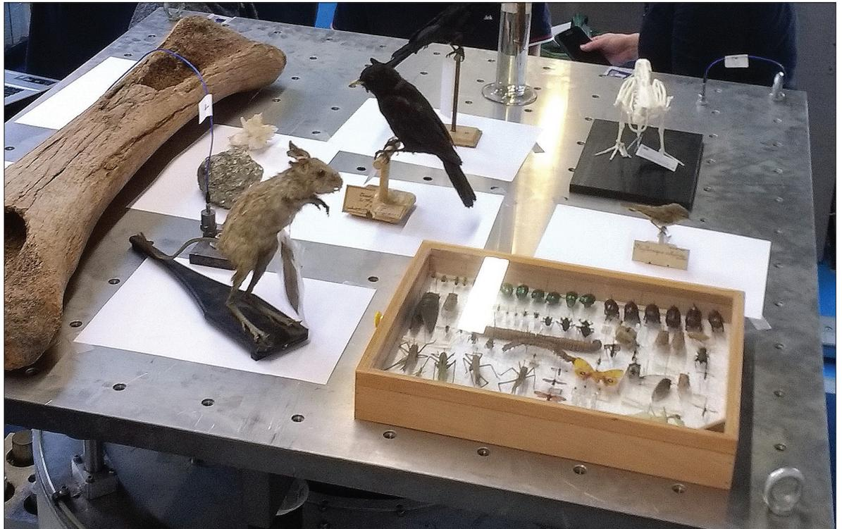
Object testing is critical for the establishment of vibration limits and mitigation methods for a “building-bound” natural-history collection.
