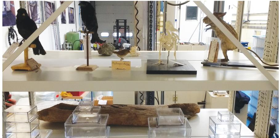
Fig. 4. Metal shelving from Naturalis being placed on the vibration table. The shelving is not fixed to the vibration table, but side beams prevent it from wandering.
