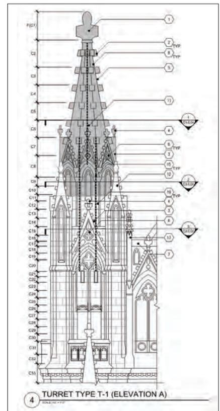
Fig. 11. Enlarged elevation of turret used in construction documents identifying course numbering and typical elements
