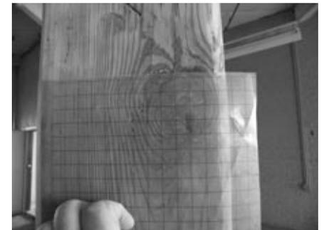
Fig. 7. The use of a 1/2-inch grid on acetate for measuring a knot on a post and timber. This knot is 1 3/4 inches in diameter.
