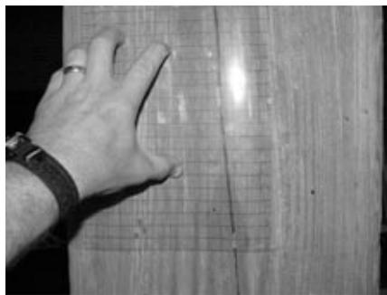
Fig. 9. The use of a  $\frac{1}{2}$ -inch grid on acetate for measuring slope of grain.
