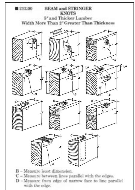
Fig. 5. Instructions for measuring knots on beams and stringers. Courtesy of Western Wood Products Association.
