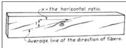
Fig. 8. Diagram showing measurement of slope of grain. Courtesy of WCLIB, Standard No. 17.
