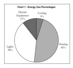
Fig. 4. Energy usage at Swift Hall broken down by building systems.
