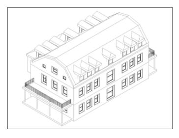
Fig. 2. An axonometric wire diagram of Swift Hall. The wire diagram allows the designer to confirm that the parameters used in the energy model match the existing conditions. Image by Bruce E. Brooks & Associates.
