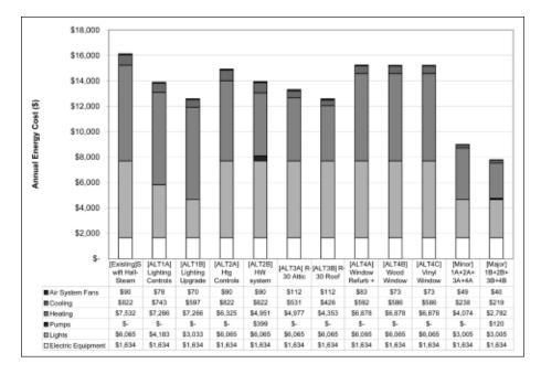
Fig. 5. Simulation results for each scenario tested using the energy model, showing not only total annual energy costs but also how each energy component of the building would be affected by the proposed change.
