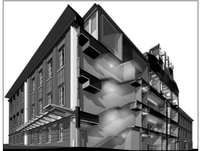
Fig. 3. James Hall, University of New Hampshire, BIM file, 2008. Overall section perspective developed for presentation, showing new addition at left, existing building rehabilitated and modified at right and beyond.
