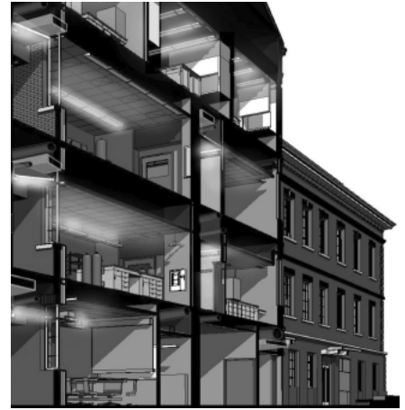
Fig. 4. Detail of Figure 3, showing (left to right) section through new corridor, laboratories, original corridor with yellow glazed brick, other spaces within, and original red brick exterior wall with steel windows, 2008.
