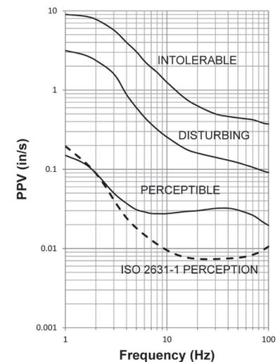
**Fig. 2. Human perceptibility of vibrations.** American Association of State Highway and Transportation Officials, R8-96, 2004; and John F. Wiss, "Construction Vibrations," (1981): 167-181.
