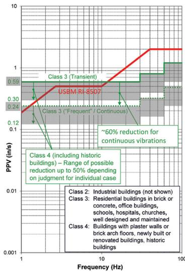
Fig. 6. Guide value vibration limits recommended by SN 640 312a for Class 3 structures, superimposed on the USBM RI 8507 limit.
