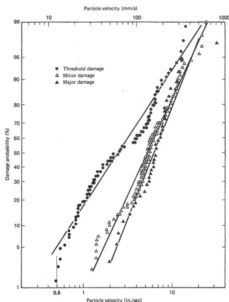
Fig. 3. Damage probability as reported in USBM RI 8507 and reproduced in C. Dowding, *Construction Vibrations*, 172.
