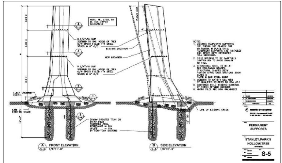
Fig. 7. Sections showing the micropiles, concrete pile cap, and major support frame, 2009. Drawing by Cascade Engineering.
