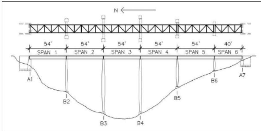
Fig. 2. Bridge arrangement, Lobato Bridge. Sketch by J. R. Harris & Co., Denver.
