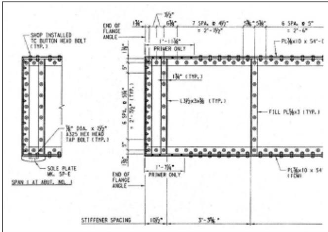
Fig. 6. Lobato Bridge, detail from the design drawings of the end of a girder. Efforts were made to replicate the historic appearance as much as possible within the confines of the project's design criteria. Compare the connections using tension controlled bolts to the original arrangement of rivets shown in Figure 3. Drawing by HDR.
