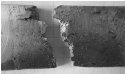
Fig. 5. Specimen, lacing bar after testing in tension failure. Photograph by the author.
