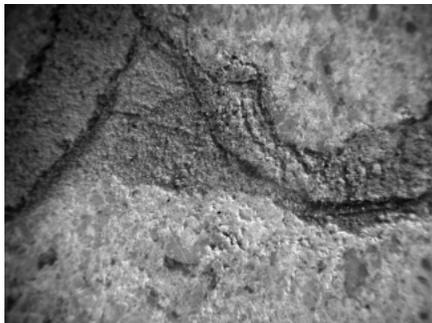
Fig. 3. The vertical surface of weathered dimensional limestone. The photograph was taken with the field microscope and camera shown in Figure 2, using natural, low-angle lighting. The width of the field of view is  $\frac{3}{16}$  inch.
