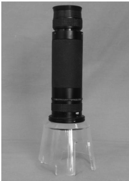
Fig. 1. A simple and effective field microscope. All images courtesy of the authors.
