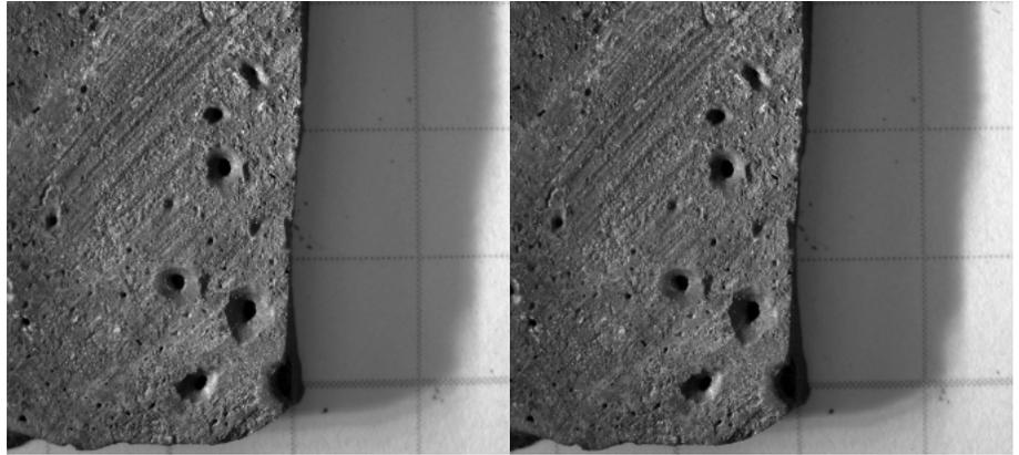
Fig. 8. Stereo images of a capping-compound fragment. Note the difference in shadow length on the right side of the fragment shown in each image, which makes it possible to determine the thickness of the fragment.
