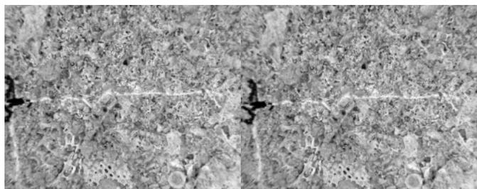
Fig. 9. Stereo images of the eroded Indiana limestone, with visible fossil fragments.
