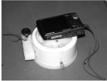
Fig. 6. The macrotube with a digital camera attached.
