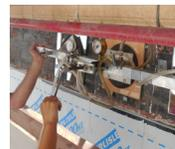
**Testing Vitrolite Adhesion:
